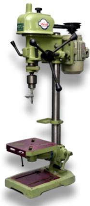
With full body part of Drillchuck, Motor, Pully, V Belt, R/F Switch.
